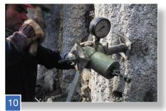
Fix the hydraulic press with a third washer plate and wing nut and then apply a load of 100kN.
